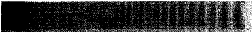
Fig. 1. Typical example of Liesegang patterns obtained with the reagents A = \text{NaOH} and B = \text{MgCl}_2 in a gel. The light grey precipitate is D = \text{Mg}(\text{OH})_2 . The experiments were carried out by M. Zrinyi (Technical University of Budapest).
